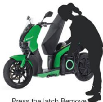
Press the latch Remove the battery pack
